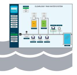
Clearlogx<sup>®</sup> controls the charge of the floc particles by ajusting coagulant based on zeta potential, pH and temperature. In conventional flocculation/sedimentation systems it improves settling and turbidity removal, reducing carryover. In membrane systems, controlling the particle charge optimizes removal of soluble organics & turbidity while reducing fouling based on electrostatic attraction.
