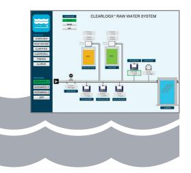
Clearlogx® controls the charge of the floc particles by ajusting coagulant based on zeta potential, pH and temperature. In conventional flocculation/sedimentation systems it improves settling and turbidity removal, reducing carryover. In membrane systems, controlling the particle charge optimizes removal of soluble organics & turbidity while reducing fouling based on electrostatic attraction.
